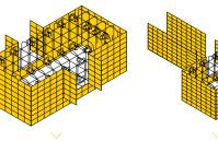
Leave top wire intact and cut alternate wires at 'door' hinge point. This helps to give a tight bend and makes the folding easier. The 'doors' act as the grout seal. Spacers may be removed at door openings.
