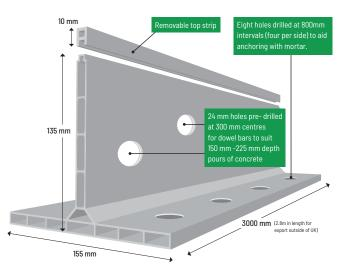
**K-FORM K35 Screed Rail** for Slab thickness 50mm - 100mm
